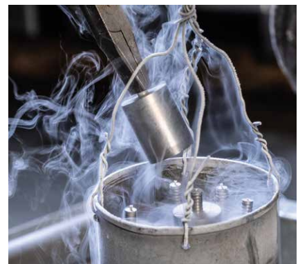
Fig. 5: Before use, a freeze-fit plug must be cooled down to -196 °C with liquid nitrogen, while the corresponding die insert must be heated to 350 °C.
